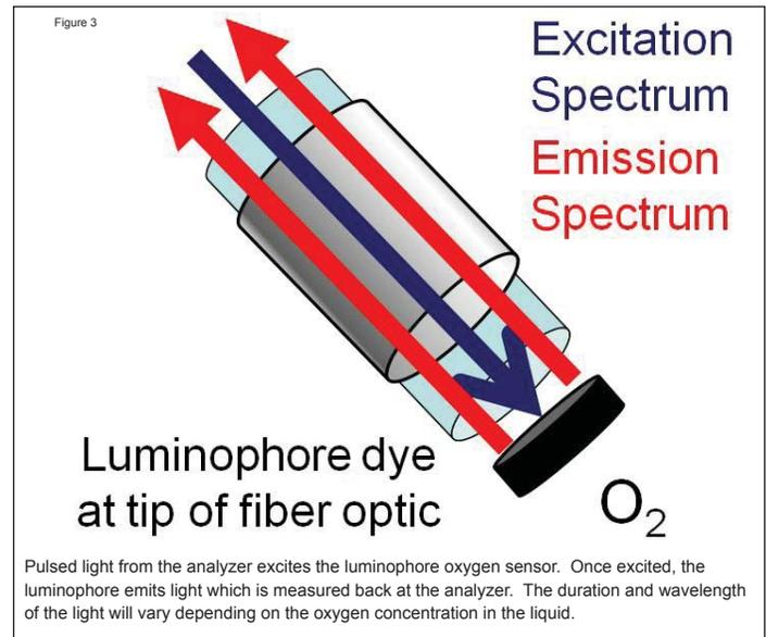
Advantages of this design include no interference due to moisture, H<sub>2</sub>S, CO<sub>2</sub>, and other contaminant gases. The 4401OXY also simplifies the sample system design as the contaminant gases do not need to be scrubbed prior to the measurement. The end result is increased reliability, better accuracy, and faster response in biogas applications.
