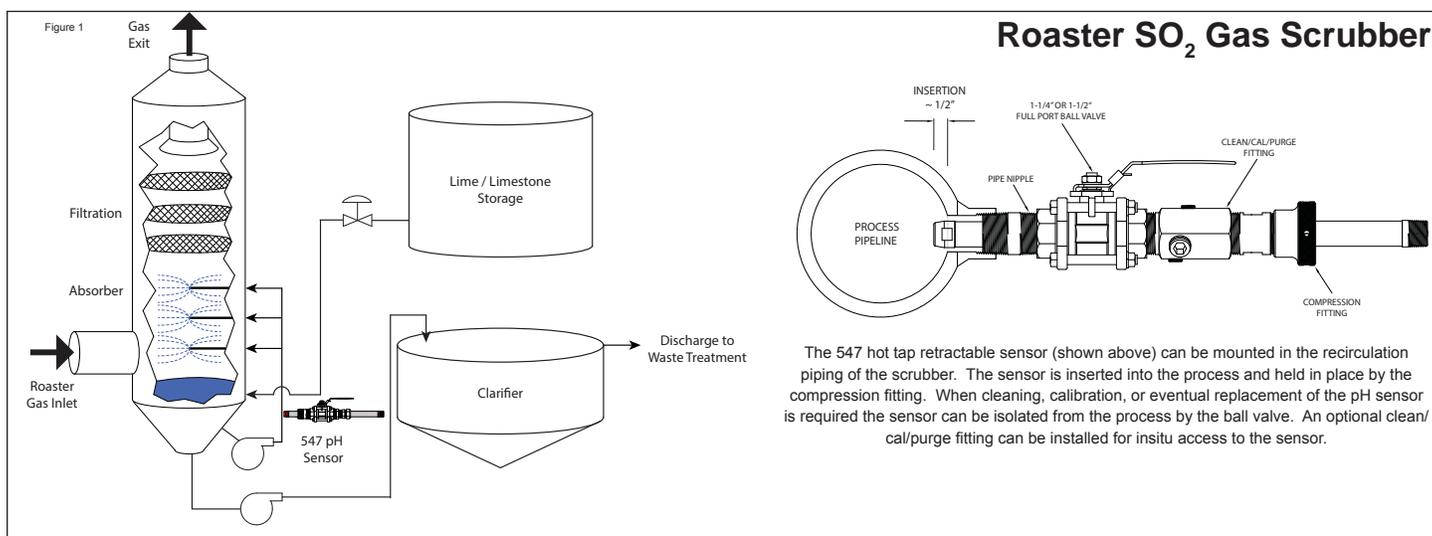
The 547 hot tap retractable sensor (shown above) can be mounted in the recirculation piping of the scrubber. The sensor is inserted into the process and held in place by the compression fitting. When cleaning, calibration, or eventual replacement of the pH sensor is required the sensor can be isolated from the process by the ball valve. An optional clean/cal/purge fitting can be installed for insitu access to the sensor.
