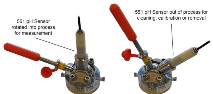
The weld pad version of the Satron PASVE Valve is shown above. The left image shows the valve with the sensor rotated into the process. The right image shows the valve when the sensor is rotated out of the process. 1/4" cleaning taps on either side of the valve allow for in situ cleaning when the sensor is retracted from the process. The PASVE valve design is well suited to the high particulate applications found in titanium dioxide production applications.
