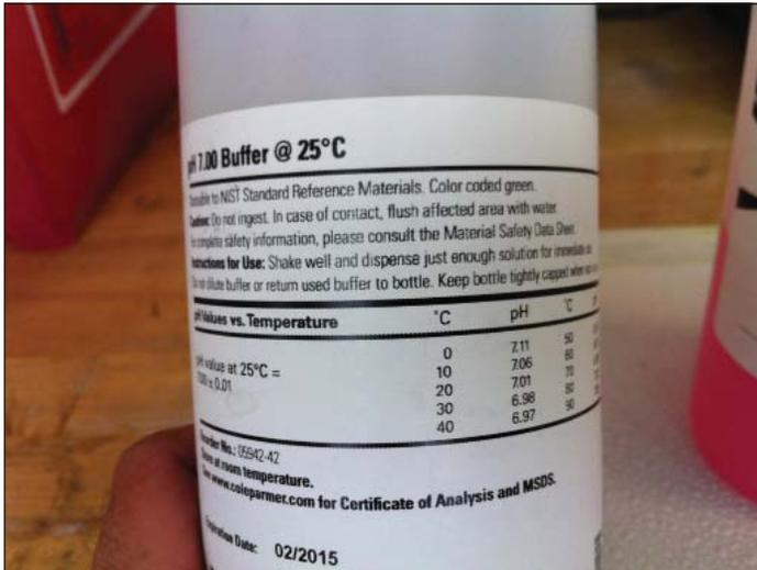
The effects of temperature on buffer solutions are highlighted on the labeling for this buffer solution.
