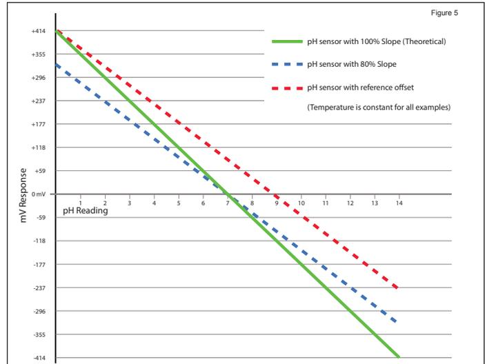
The above graph shows the effect of slope and offset on the sensor response. The blue line shows how a sensor with 80% slope puts out less mV's per a given pH value than a new sensor (represented by green line). This can be corrected via a two point buffer calibration.
